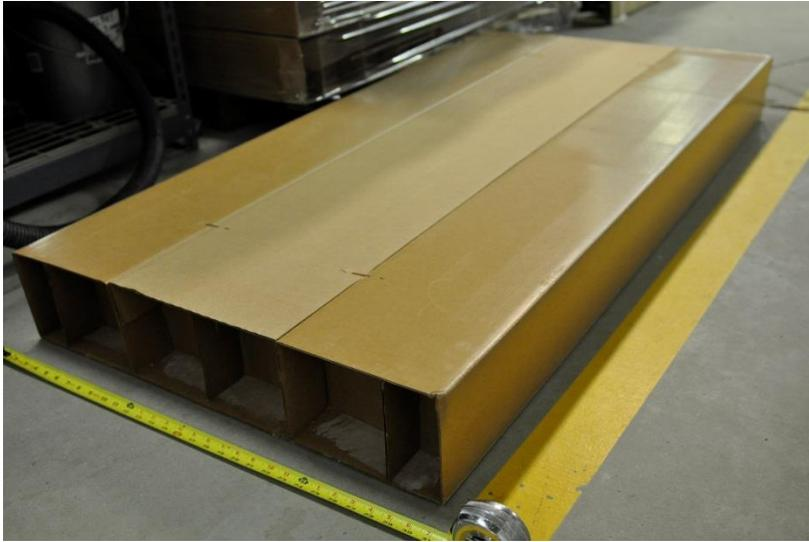
*Figure 3. Cardboard void slab form*
