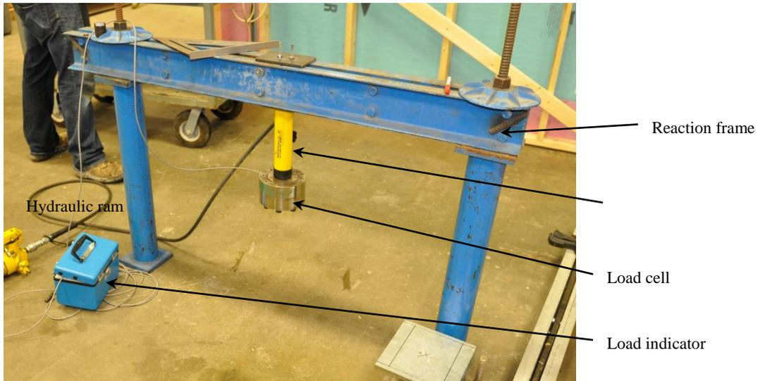
Figure 5. Typical test setup
