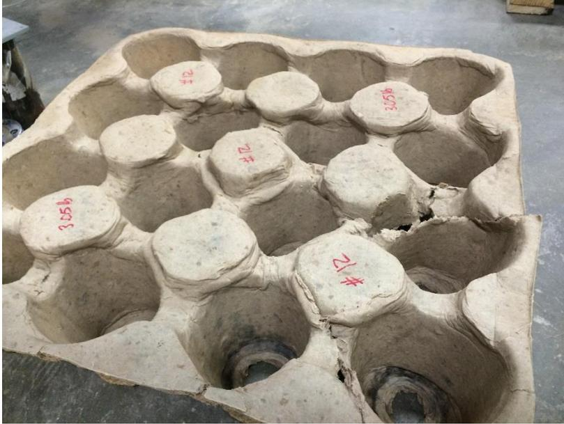
*Figure 9. Failure of a molded pulp void form*
