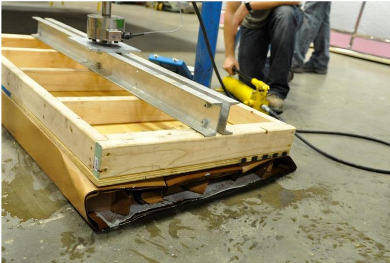
*Figure 8. Failure of a slab cardboard void form*
