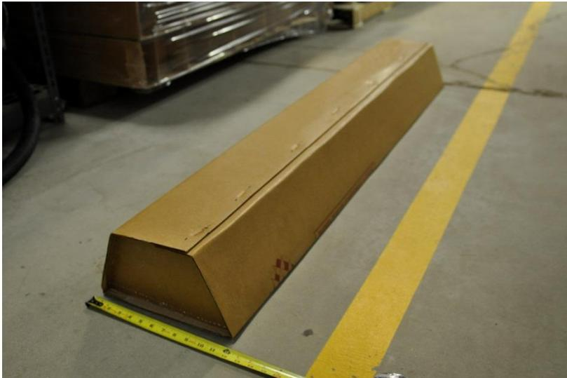
*Figure 2. Cardboard void trap form*
