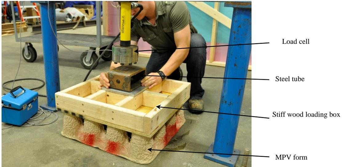
*Figure 7. Typical MPV form*
