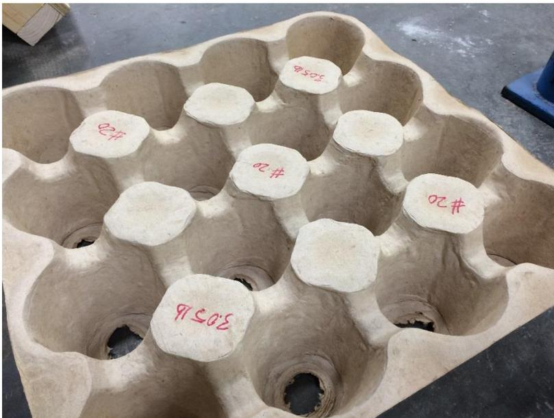
*Figure 4. Molded pulp void form*
